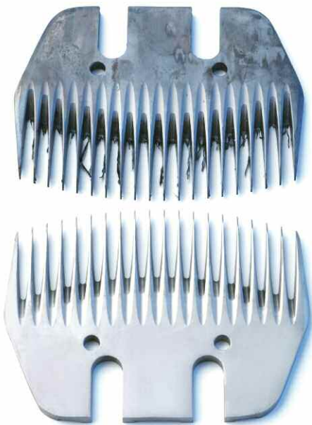
Carbon steel hair clipper blade untreated, FerroChem-treated
