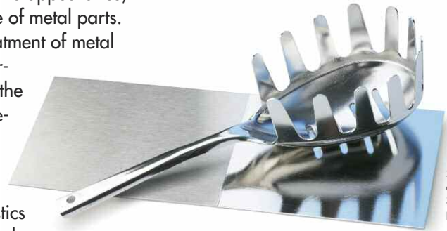
Spaghetti-gripper on a stainless steel sheet Stainless steel sheet partly electro polished
